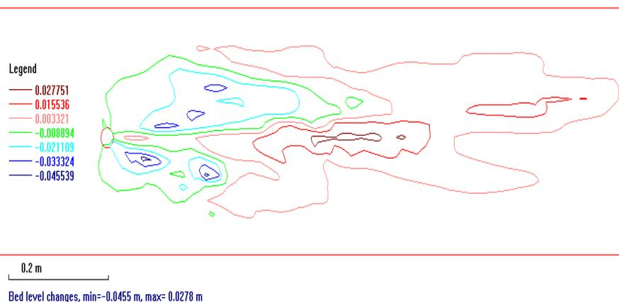
**Figure 2. Scour around the pier after 7 hours in the calibrated SSIIM model.**
