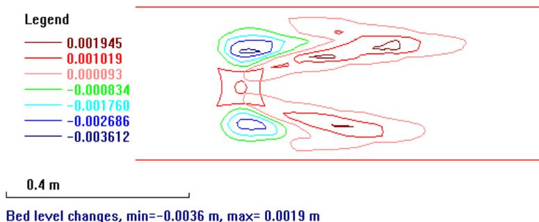
Figure 4. Contours of bed level around the bridge pier with the collar precisely installed at bed level.
