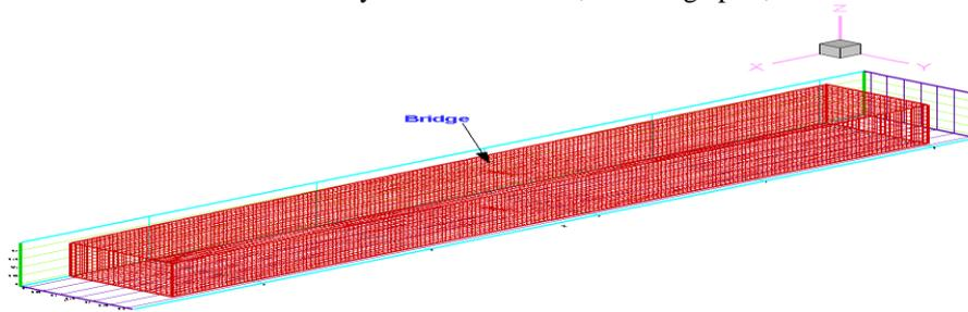
Figure 1. The final calculation mesh of the canal encapsulating the pier.
