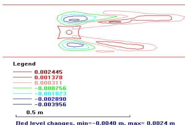
Figure 5. Contours of bed level around the bridge pier with a collar in place above bed level 0.2 times the water depth.
