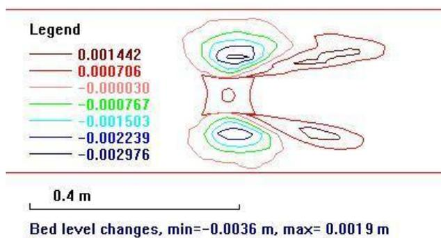
Figure 6. Contours of bed level around the bridge pier with a collar bed level 0.2 times the water depth.
