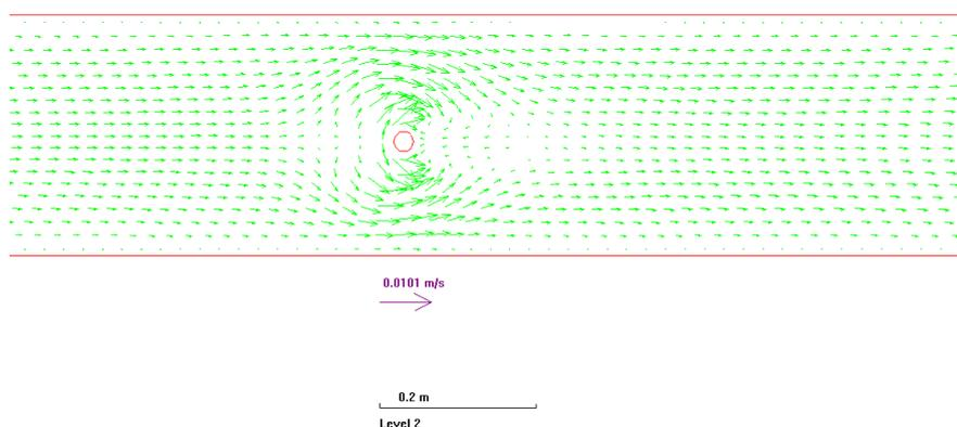
**Figure 3. Magnified velocity vectors of the flow field around the pier in the bed after simulation (no collar installed).**
